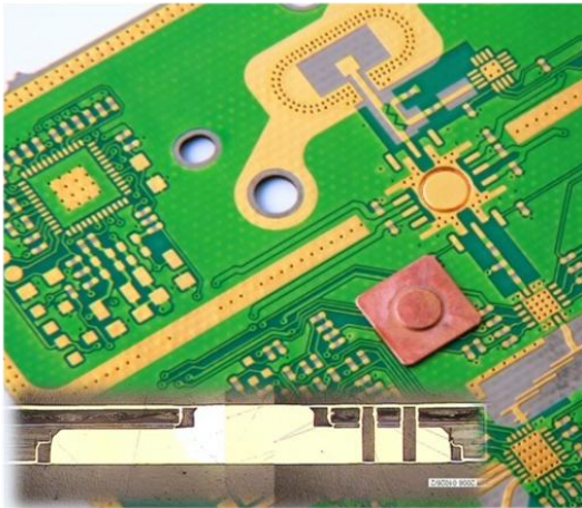
Figure 6. PCB with embedded copper coin
